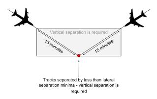
Vertical separation is no longer required once both aircraft have passed each other by:
