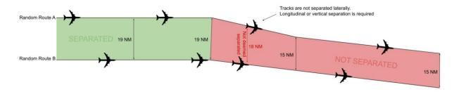
In Figure 2, aircraft A and B are laterally separated for the first portion of their route (green), however lateral separation does not exist once aircraft A's track deviates south. As soon as the first aircraft reaches the route portion that is no longer laterally separated, separation is lost. Therefore, another form of separation must be in place and separation ensured <u>before this point is reached by either aircraft.</u>
