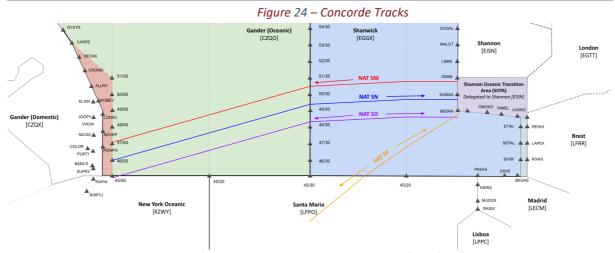
**Note:** Supersonic flight on Concorde tracks is separated from flights via other Concorde tracks.
